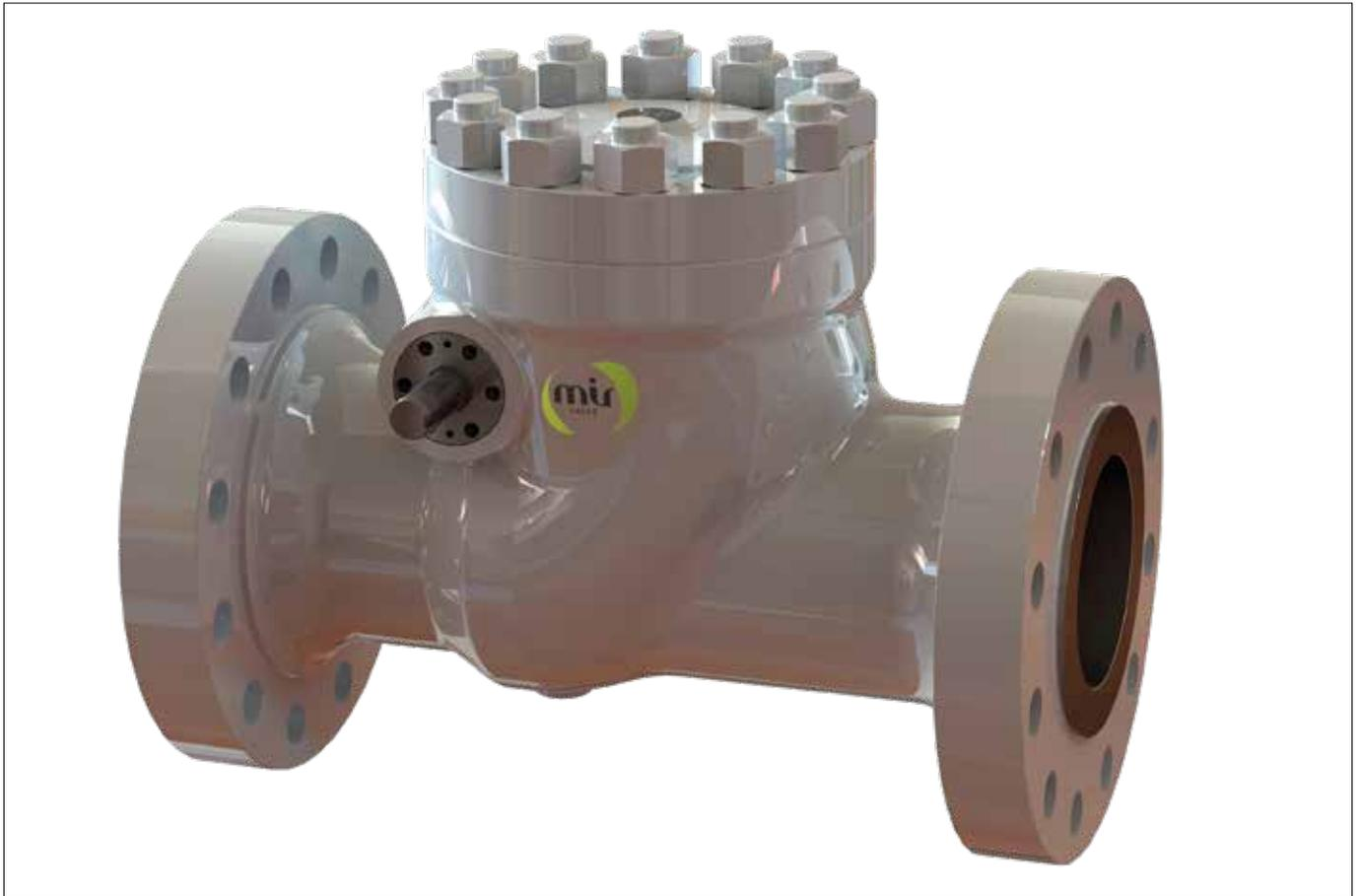
The purpose of a swing check valve is to prevent fluid flow from travelling in the upstream direction. A swing check valve fulfills this purpose by letting a hinged clapper shut against the seat.
